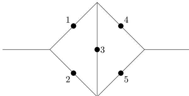
Figure 2.1.4: Pictorial representation of a bridge system.
