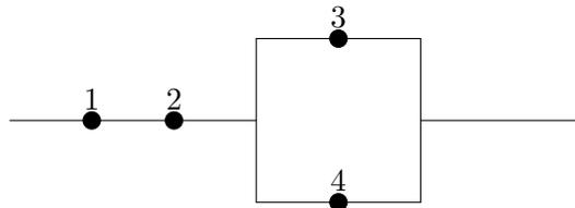
Figure 2.1.3: Pictorial representation of a four-component hybrid system.
