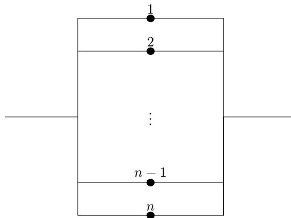
Figure 2.1.2: Pictorial representation of an  $n$ -component parallel system.
